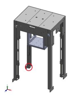
Using socket driver with 3/16" inch socket attached, loosen nuts on lower flexures while counter holding bolts using ½" box end wrench. Remove nuts, bolts, and the lower flat bracket from the pendulum arm.
