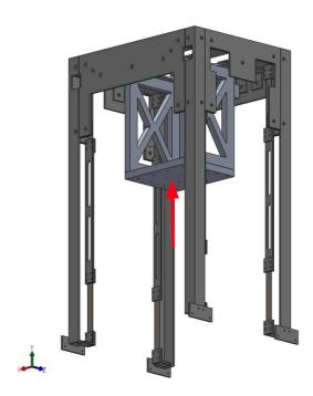
4. While supporting the shelf from step 3, remove 4 bolts, indicated in red circles below, securing the thruster shelf to the pendulum using a socket driver with a 5/16" socket.
