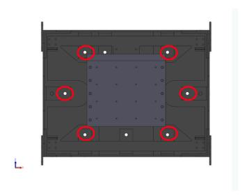
Remove panels from the pendulum frame.
