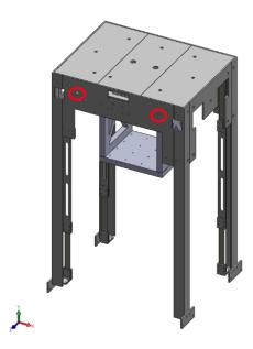
2. Once the pendulum top is supported, access bolts through cut out, indicated in red circles below, using a size PH1 phillips head screwdriver.
