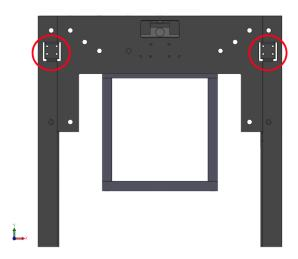
Access the nuts on the other side of the pendulum arm through the cut outs indicated with red circles below. Using a ¼" box end wrench to counter hold the nuts, fully loosen each bolt using the screwdriver. Remove each nut, but leave bolts and the upper flat bracket in place to keep the pendulum arm supported.
