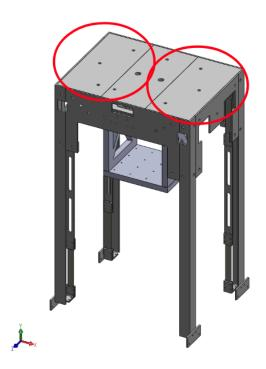
Bolts can be accessed from top using a  $\frac{3}{8}$ " box end wrench. The nuts are accessed from below, indicated below, using a socket driver with a 7/16" socket attached.
