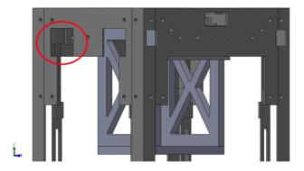
3. At lower flexure access nuts and bolts on corner bracket indicated below in red circles
