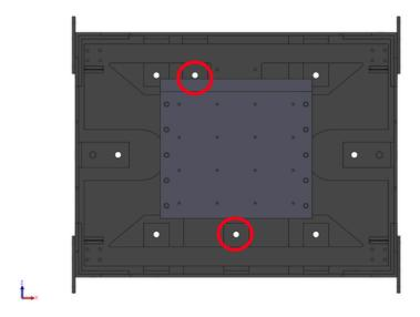
2. Remove side panels on top of pendulum frame, indicated in red circles below.
