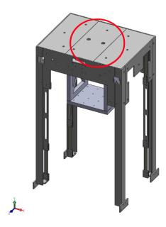
Bolts can be accessed from top using a 3/8" box end wrench. The nuts are accessed from below, indicated below, using a socket driver with a 7/16" socket attached. Using 1/2" holes in the center of the panel to remove the panel.
